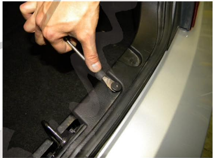
2. Remove the (6) plastic clips
