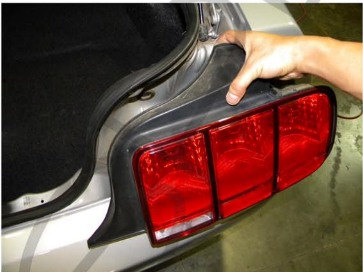
9. Remove the stock tail light
