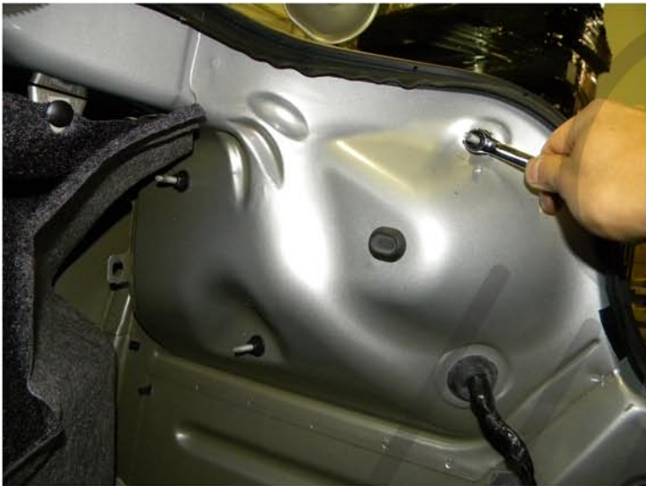
7. Remove the (3) 10mm nuts
