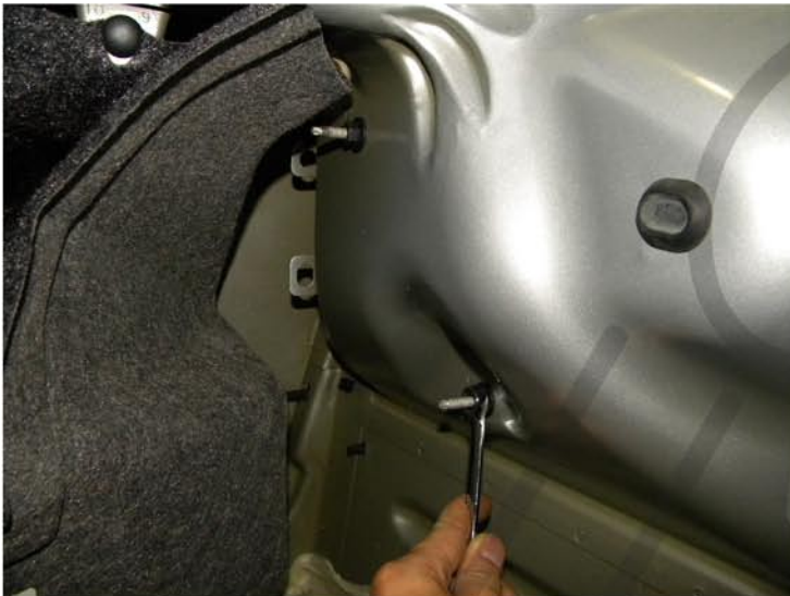
13. Tighten (3) 10mm bolts
