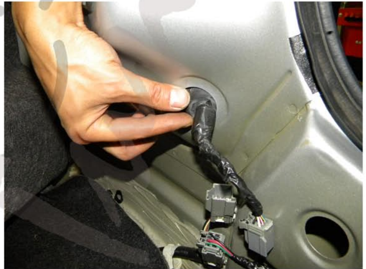
8. Push in the harness rubber seal
