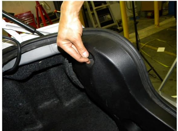
4. Remove the (6) plastic clips
