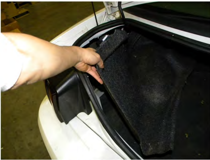
17. Replace the side trunk liner
