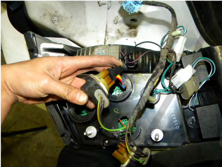
13. Plug the tail light harness into the LED tail light
