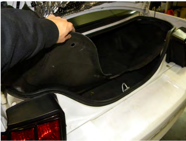
5. Remove the rear trunk liner
