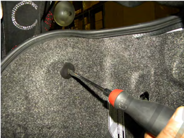
19. Tighten the plastic flat head clip
