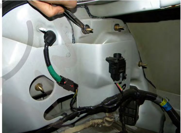
8. Remove the (4) 11mm nuts
