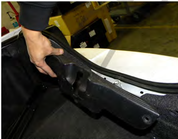
3. Remove the plastic moulding
