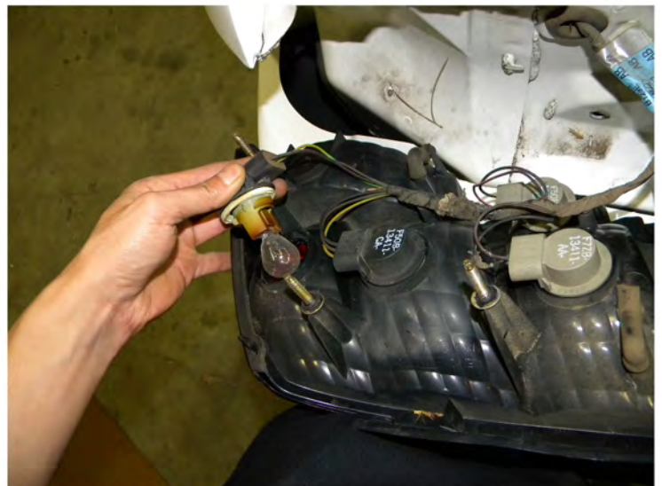
10. Remove the light harness and the bulbs
