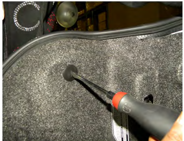
4. Remove the plastic flat head clip
