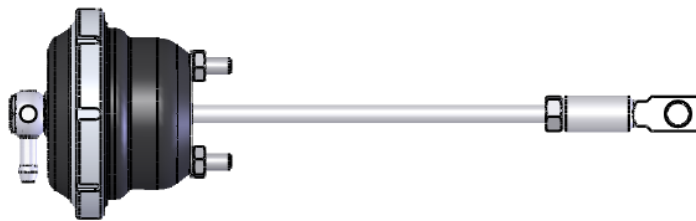
IWG75 with Ø8.2mm clevis
