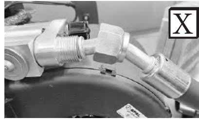
Improperly Seated O-ring Land
