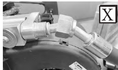
Improperly Seated O-ring Land
