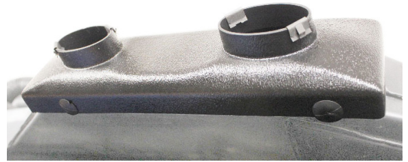
Photo 15 - Install Defrost Duct
