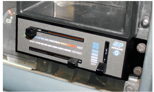
Photo 20 - Install Wire Harness and Control
